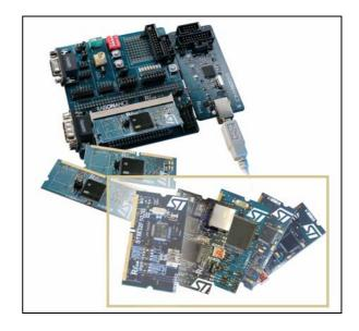
evaluation board, microcontrollers, embedded RLink JTAG in-circuit debugger/programmer and Raisonance Integrated Development Environment (RIDE).
